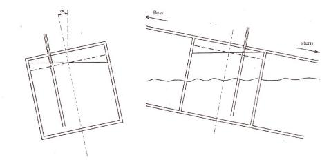
The volume is obtained after applying an LNG temperature correction to the value taken from the gauging tables so that the contraction factor of the tank's walls is accounted for.
